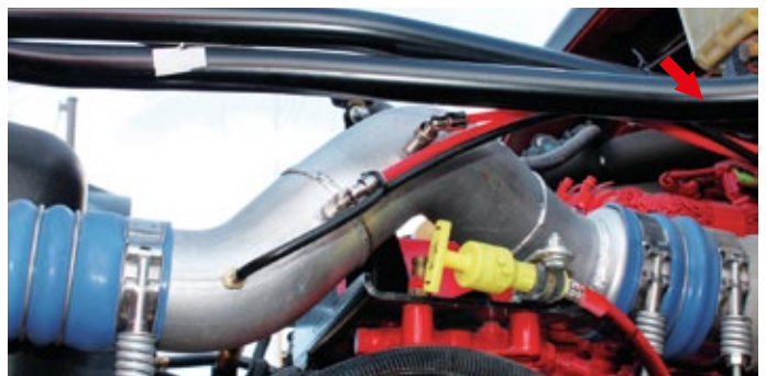
Mounting example 8.3l Cummins Diesel. Boost source adapter (left) und 2 installed nozzles.
