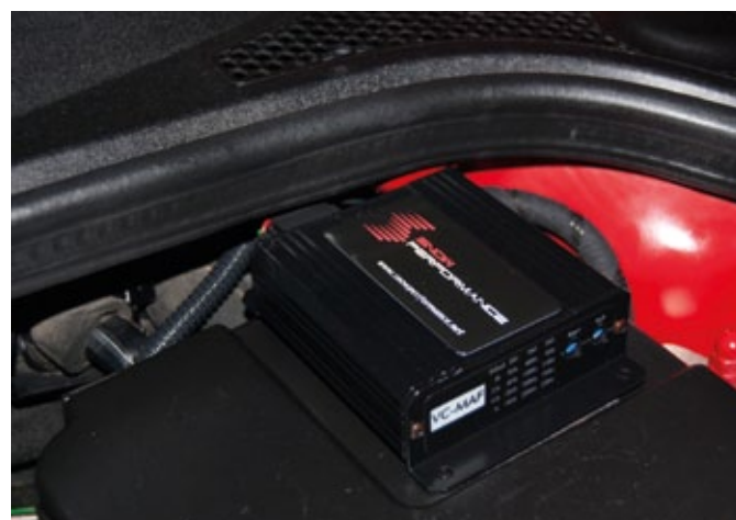
Audi A3 2.0TFSI with Boost Cooler controller within the engine compartment
