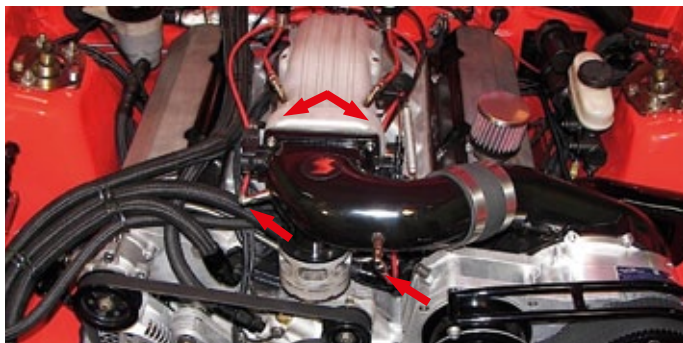
NASCAR engine (<1200 hp) with Boost Cooler
