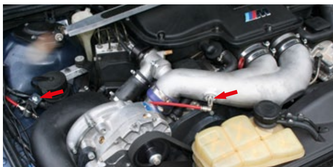
Supercharged BMW M5 with Boost Cooler Stage 2 and installed solenoid (left)
