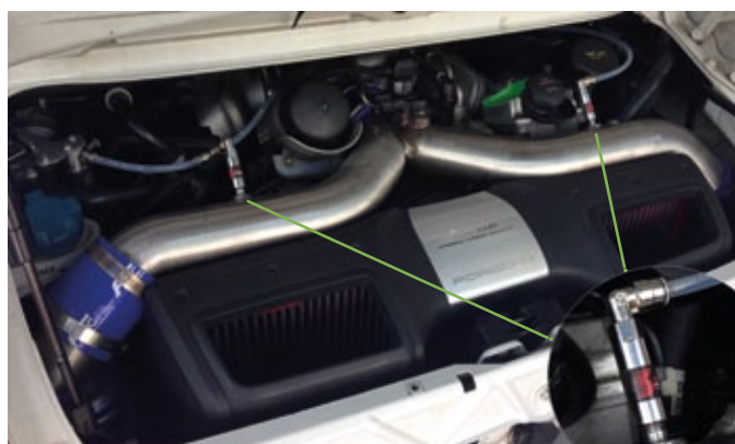
Mounting Example Porsche 997 Turbo with Dual Nozzle
