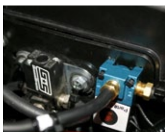
Mounting Example Mazda 3 (SI-Solenoid)
